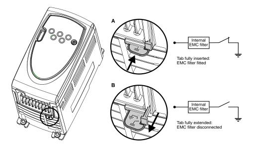
Commander SK A thru D uses pull tab
