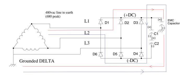
In the grounded wye connection shown below, the same process occurs with the exception that the peak voltage with respect to earth ground is only 390 volts instead of the 680 volts as above. In this case the energy transferred will not be enough to cause the dc bus to charge to the over voltage trip level.
