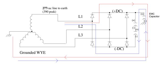
The other two configurations, ungrounded Delta and Wye connections do not typically exhibit the over voltage charging. In rare cases if the coupling capacitance to earth ground in the power system is unusually high on one phase a charging path could be created. In this case, (in fact any configuration other than grounded Wye) the capacitor should be removed.
