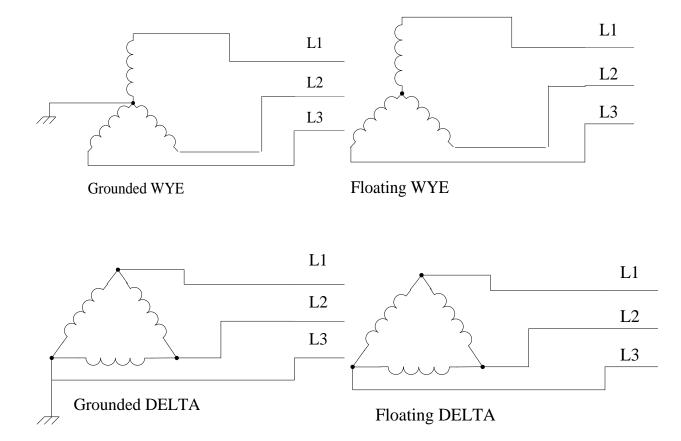
These transformer configurations feed 3 phase power to our drive's "rectifier front end" as shown below. As can be seen, the 3 phase rectifier feeds a DC bus with the EMC filter providing a high frequency shunt path from DC+ to Earth.
